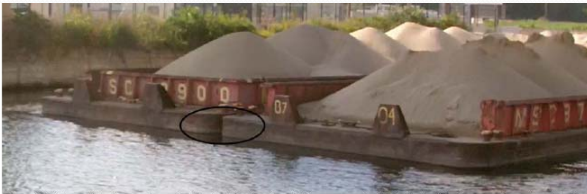
Figure 12. Picture of two barges traversing the electrical barrier with the square ends in the front of the barge configuration. The circle denotes the small void space that two live fish swam into and became entrained past the barrier.
